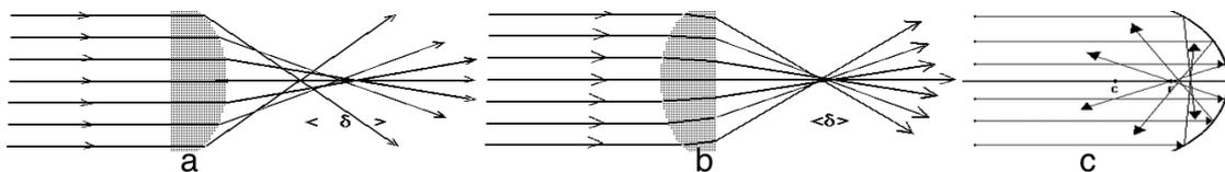
Figure 1: Spherical Aberration of Planoconvex Lens With Collimated Beam. [3]
