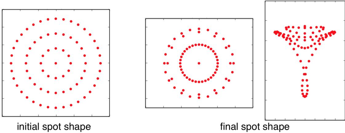
Figure 2: Spherical Aberration And Coma Aberration.
